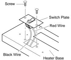
Figure 27 - Switch Plate and Wiring Harness
